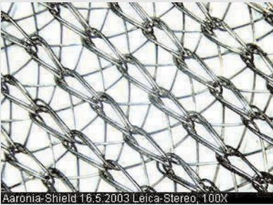
The elaborate high-tech weaving technique of Aaronia-Shield® offers the best shielding values possible, especially in high GHz ranges.
