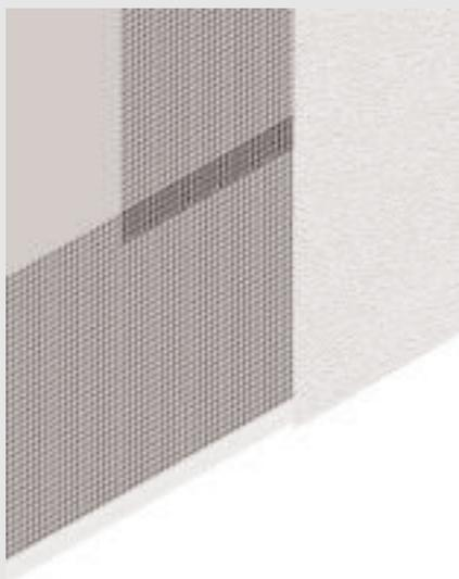
In order to achieve protection of a room, for example the bedroom, against high-frequency radiation, the room must be completely lined with Aaronia X-Dream® .
