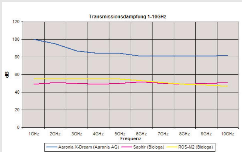
Standardized readings according to MIL-STD-285 attest the extremely high level of shielding of Aaronia X-Dream®: Reduction/attenuation of high-frequency radiation, especially in the frequency range that is subject to pulsed signals from mobile phone stations, is 80dB (99.999.999.99%).
