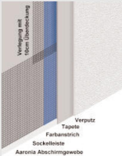
Houses and buildings under construction should always be shielded on the exterior.
