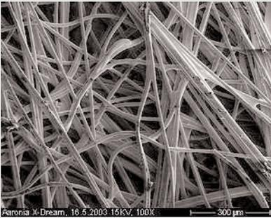
Electron microscope scans show that the individual fibers are inseparably fused to form an impenetrable structure against HF radiation.
